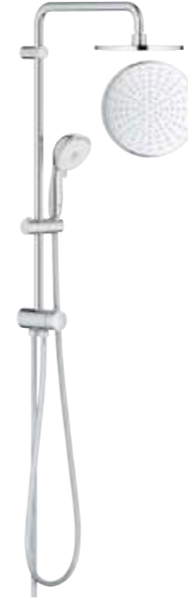
27 399 002 New Tempesta Rustic System 200 Flex shower system with diverter Distance between diverter and upper bracket: 620 mm hand shower 4-sprays 390 mm shower arm
